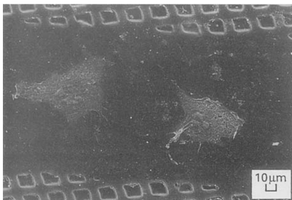
Figure 7 SEM of fibroblasts on PEI 7 μm pillars with 5 pulses (2.5 μm deep).
